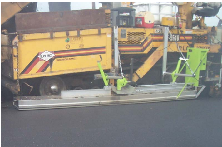
Fusion PM shown mounted on a paver
