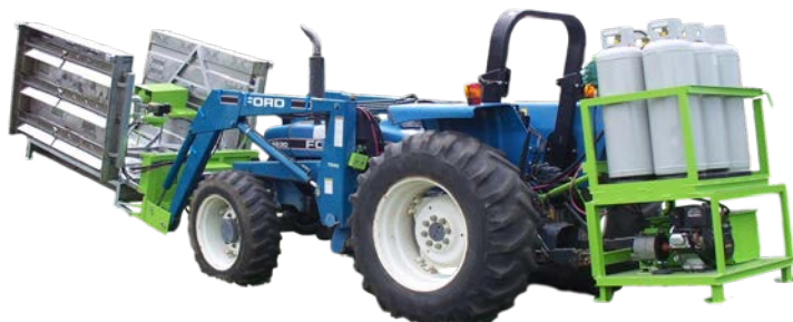
Tech 78 (Folding chamber - Total size 6'L x 13'W)
