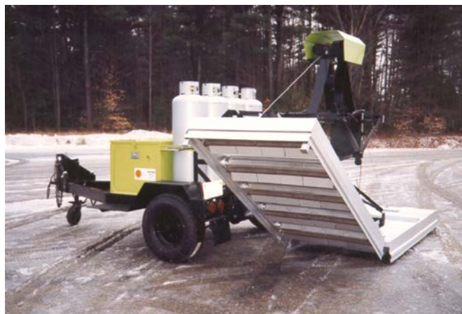
Tech 36 (bi-fold chamber 3'L x 13'W total)
