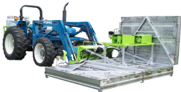
Tech 78 (Folding chamber - Total size 6'L x 13'W)
